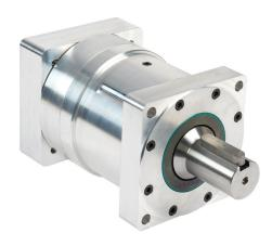
SureGear high-precision strain wave gearbox, 50:1 ratio, inline, 32mm diameter output shaft, nominal output torque 100 N-m (885 lb-in), 1-stage, 116mm frame. For use with SureServo and SureServo2 SV(2)L-210(B) motors.
