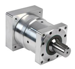
SureGear high-precision strain wave gearbox, 200:1 ratio, inline, 32mm diameter output shaft, nominal output torque 120 N-m (1062 lb-in), 1-stage, 116mm frame. For use with SureServo SVM-210(B) motors.
