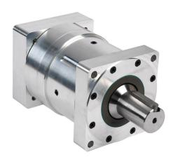
SureGear high-precision strain wave gearbox, 200:1 ratio, inline, 32mm diameter output shaft, nominal output torque 120 N-m (1062 lb-in), 1-stage, 116mm frame. For use with SureServo and SureServo2 SV(2)L-210(B) motors.
