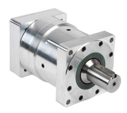
SureGear high-precision strain wave gearbox, 160:1 ratio, inline, 32mm diameter output shaft, nominal output torque 120 N-m (1062 lb-in), 1-stage, 116mm frame. For use with SureServo and SureServo2 SV(2)L-210(B) motors.
