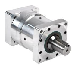
SureGear high-precision strain wave gearbox, 135:1 ratio, inline, 32mm diameter output shaft, nominal output torque 120 N-m (1062 lb-in), 1-stage, 116mm frame. For use with SureServo and SureServo2 SV(2)L-210(B) motors.
