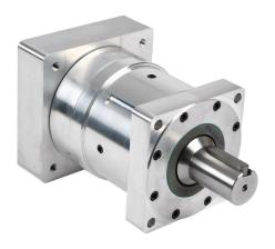
SureGear high-precision strain wave gearbox, 100:1 ratio, inline, 32mm diameter output shaft, nominal output torque 120 N-m (1062 lb-in), 1-stage, 116mm frame. For use with SureServo SVM-210(B) motors.
