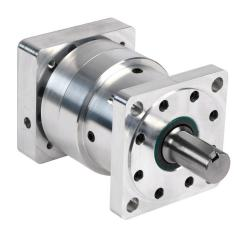
SureGear high-precision strain wave gearbox, 80:1 ratio, inline, 22mm diameter output shaft, nominal output torque 40 N-m (354 lb-in), 1-stage, 88mm frame. For use with SureServo and SureServo2 SV(2)L-207(B) motors.
