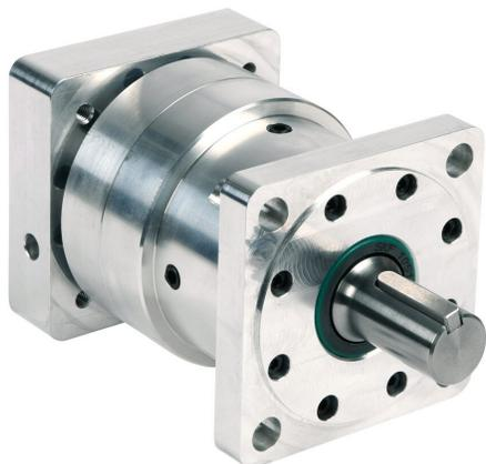
SureGear high-precision strain wave gearbox, 50:1 ratio, inline, 22mm diameter output shaft, nominal output torque 40 N-m (354 lb-in), 1-stage, 88mm frame. For use with SureServo and SureServo2 SV(2)L-207(B) motors.
