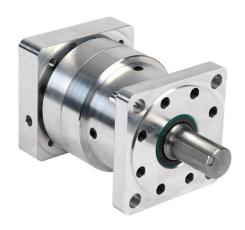
SureGear high-precision strain wave gearbox, 120:1 ratio, inline, 22mm diameter output shaft, nominal output torque 50 N-m (443 lb-in), 1-stage, 88mm frame. For use with SureServo and SureServo2 SV(2)L-207(B) motors.
