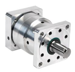
SureGear high-precision strain wave gearbox, 100:1 ratio, inline, 22mm diameter output shaft, nominal output torque 50 N-m (443 lb-in), 1-stage, 88mm frame. For use with SureServo and SureServo2 SV(2)L-207(B) motors.
