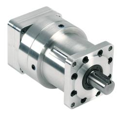
SureGear high-precision strain wave gearbox, 50:1 ratio, inline, 16mm diameter output shaft, nominal output torque 25 N-m (221 lb-in), 1-stage, 73mm frame. For use with SureServo and SureServo2 SV(2)L-202(B) and SV(2)L-204(B) motors.
