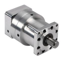
SureGear high-precision strain wave gearbox, 100:1 ratio, inline, 16mm diameter output shaft, nominal output torque 30 N-m (266 lb-in), 1-stage, 73mm frame. For use with SureServo and SureServo2 SV(2)L-202(B) and SV(2)L-204(B) motors.
