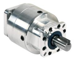
SureGear high-precision strain wave gearbox, 50:1 ratio, inline, 13mm diameter output shaft, nominal output torque 12 N-m (106 lb-in), 1-stage, 63mm frame. For use with SureServo and SureServo2 SV(2)L-201(B) motors.
