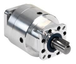
SureGear high-precision strain wave gearbox, 100:1 ratio, inline, 13mm diameter output shaft, nominal output torque 15 N-m (133 lb-in), 1-stage, 63mm frame. For use with SureServo and SureServo2 SV(2)L-201(B) motors.
