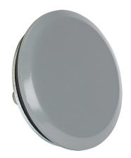
Hammond hole seal, 30mm pushbutton, carbon steel, ANSI 61 gray, powder coat finish, oil-resistant gasket. For use with carbon steel enclosures.
