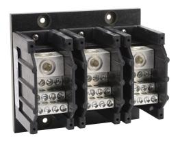
Edison open power distribution block, 310A, 3-pole, line side: 1 opening accepts 350 MCM to 4 AWG, load side: 12 openings accept 4AWG to 14 AWG, panel mount, UL 1953 listed.
