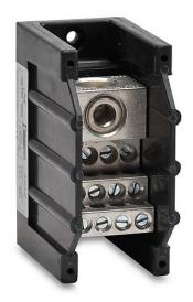
Edison open power distribution block, 310A, 1-pole, line side: 1 opening accepts 350 MCM to 4 AWG, load side: 12 openings accept 4AWG to 14 AWG, panel mount, UL 1953 listed.
