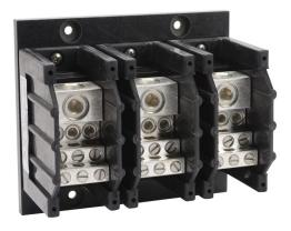
Edison open power distribution block, 310A, 3-pole, line side: 1 opening accepts 350 MCM to 4 AWG, load side: 6 openings accept 2AWG to 12 AWG, 3 openings accept 1/0 to 12 AWG, panel mount, UL 1953 listed.
