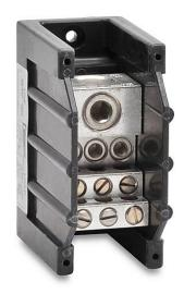
Edison open power distribution block, 310A, 1-pole, line side: 1 opening accepts 350 MCM to 4 AWG, load side: 6 openings accept 2AWG to 12 AWG, 3 openings accept 1/0 to 12 AWG, panel mount, UL 1953 listed.
