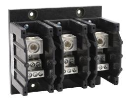
Edison open power distribution block, 310A, 3-pole, line side: 1 opening accepts 350 MCM to 4 AWG, load side: 6 openings accept 4 AWG to 12 AWG, panel mount, UL 1953 listed.
