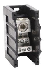
Edison open power distribution block, 310A, 1-pole, line side: 1 opening accepts 350 MCM to 4 AWG, load side: 6 openings accept 4 AWG to 12 AWG, panel mount, UL 1953 listed.
