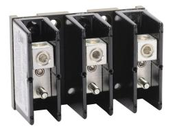
Edison open power distribution block, 175A, 3-pole, line side: 1 opening accepts 2/0 AWG to 8 AWG, load side: 1/4-20 X 3/4 stud, panel mount, UL 1953 listed.
