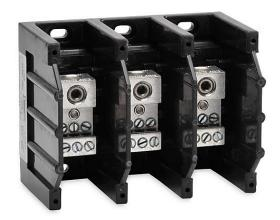
Edison open power distribution block, 175A, 3-pole, line side: 1 opening accepts 2/0 AWG to 8 AWG, load side: 6 openings accept 4 AWG to 14 AWG, panel mount, UL 1953 listed.
