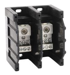
Edison open power distribution block, 175A, 2-pole, line side: 1 opening accepts 2/0 AWG to 8 AWG, load side: 6 openings accept 4 AWG to 14 AWG, panel mount, UL 1953 listed.
