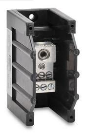
Edison open power distribution block, 175A, 1-pole, line side: 1 opening accepts 2/0 AWG to 8 AWG, load side: 6 openings accept 4 AWG to 14 AWG, panel mount, UL 1953 listed.
