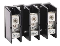
Edison open power distribution block, 175A, 3-pole, line side: 1 opening accepts 2/0 AWG to 8 AWG, load side: 4 openings accept 4AWG to 14 AWG, panel mount, UL 1953 listed.
