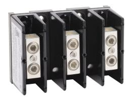
Edison open power distribution block, 175A, 3-pole, line side: 1 opening accepts 2/0 AWG to 8 AWG, load side: 1 opening accepts 2/0 AWG to 8 AWG, panel mount, UL 1953 listed.
