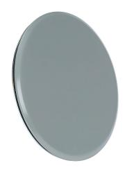
Hammond hole seal, 3-1/2in conduit, carbon steel, ANSI 61 gray, powder coat finish, oil-resistant gasket. For use with carbon steel enclosures.
