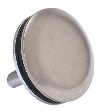
Hammond hole seal, 22mm pushbutton, 304 stainless steel, #4 brush finish, oil-resistant gasket. For use with stainless steel enclosures.
