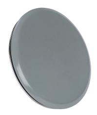
Hammond hole seal, 2in conduit, carbon steel, ANSI 61 gray, powder coat finish, oil-resistant gasket. For use with carbon steel enclosures.
