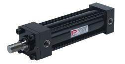
Peninsular hydraulic cylinder, NFPA tie rod, 2-1/2in bore, 1-3/8in rod diameter, 8in stroke, double acting, tapped end caps mount.
