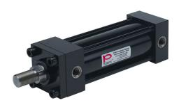
Peninsular hydraulic cylinder, NFPA tie rod, 2-1/2in bore, 1-3/8in rod diameter, 6in stroke, double acting, tapped end caps mount.
