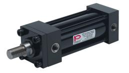
Peninsular hydraulic cylinder, NFPA tie rod, 2-1/2in bore, 1-3/8in rod diameter, 5in stroke, double acting, tapped end caps mount.
