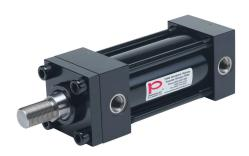
Peninsular hydraulic cylinder, NFPA tie rod, 2-1/2in bore, 1-3/8in rod diameter, 4in stroke, double acting, tapped end caps mount.
