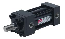
Peninsular hydraulic cylinder, NFPA tie rod, 2-1/2in bore, 1-3/8in rod diameter, 3in stroke, double acting, tapped end caps mount.
