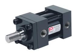
Peninsular hydraulic cylinder, NFPA tie rod, 2-1/2in bore, 1-3/8in rod diameter, 1in stroke, double acting, tapped end caps mount.
