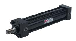
Peninsular hydraulic cylinder, NFPA tie rod, 2-1/2in bore, 1-3/8in rod diameter, 12in stroke, double acting, tapped end caps mount.
