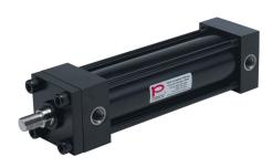
Peninsular hydraulic cylinder, NFPA tie rod, 2-1/2in bore, 1in rod diameter, 8in stroke, double acting, tapped end caps mount.
