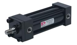
Peninsular hydraulic cylinder, NFPA tie rod, 2-1/2in bore, 1in rod diameter, 6in stroke, double acting, tapped end caps mount.
