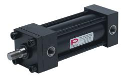
Peninsular hydraulic cylinder, NFPA tie rod, 2-1/2in bore, 1in rod diameter, 5in stroke, double acting, tapped end caps mount.
