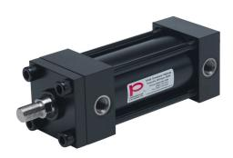
Peninsular hydraulic cylinder, NFPA tie rod, 2-1/2in bore, 1in rod diameter, 4in stroke, double acting, tapped end caps mount.
