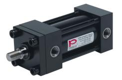
Peninsular hydraulic cylinder, NFPA tie rod, 2-1/2in bore, 1in rod diameter, 3in stroke, double acting, tapped end caps mount.
