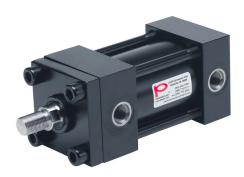
Peninsular hydraulic cylinder, NFPA tie rod, 2-1/2in bore, 1in rod diameter, 2in stroke, double acting, tapped end caps mount.
