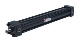
Peninsular hydraulic cylinder, NFPA tie rod, 2-1/2in bore, 1in rod diameter, 20in stroke, double acting, tapped end caps mount.
