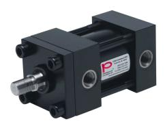
Peninsular hydraulic cylinder, NFPA tie rod, 2-1/2in bore, 1in rod diameter, 1in stroke, double acting, tapped end caps mount.
