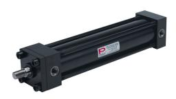
Peninsular hydraulic cylinder, NFPA tie rod, 2-1/2in bore, 1in rod diameter, 12in stroke, double acting, tapped end caps mount.
