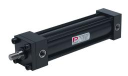
Peninsular hydraulic cylinder, NFPA tie rod, 2-1/2in bore, 1in rod diameter, 10in stroke, double acting, tapped end caps mount.
