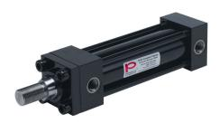
Peninsular hydraulic cylinder, NFPA tie rod, 2in bore, 1-3/8in rod diameter, 6in stroke, double acting, tapped end caps mount.
