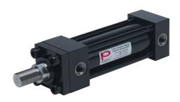
Peninsular hydraulic cylinder, NFPA tie rod, 2in bore, 1-3/8in rod diameter, 5in stroke, double acting, tapped end caps mount.
