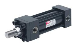
Peninsular hydraulic cylinder, NFPA tie rod, 2in bore, 1-3/8in rod diameter, 4in stroke, double acting, tapped end caps mount.
